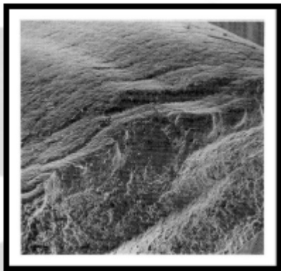
Fracture surface of Geller Spoon magnified up to 50 times.
